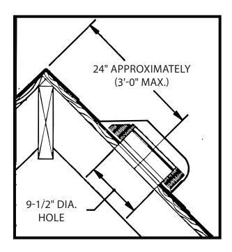
5. Starting in the drill holes cut two 9-1/2" diameter circular openings, using either a keyhole saw or an electric saber saw with sharp coarse blade. If you do not have a coarse blade, cut away shingles inside the circle with utility knife before cutting roof decking. Take care not to make the holes too large or water leakage may occur.
