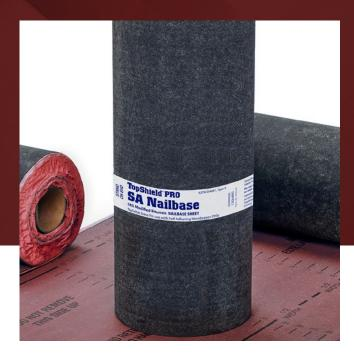
**TopShield® PRO SA NailBase** is designed for use as an anchor sheet in self-adhering roofing systems. It is suitable for use in the construction of various types of membranes for both new construction and reroofing over a variety of substrates. TopShield®PRO SA NailBase permits complete mechanical attachment to nailable substrates, preserving the integrity of the substrate for future tear-offs and adding additional waterproofing performance capabilities to the overall system.
